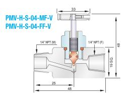
PANAM Mini Series Needle Valves are also available in Female to Female end connections
